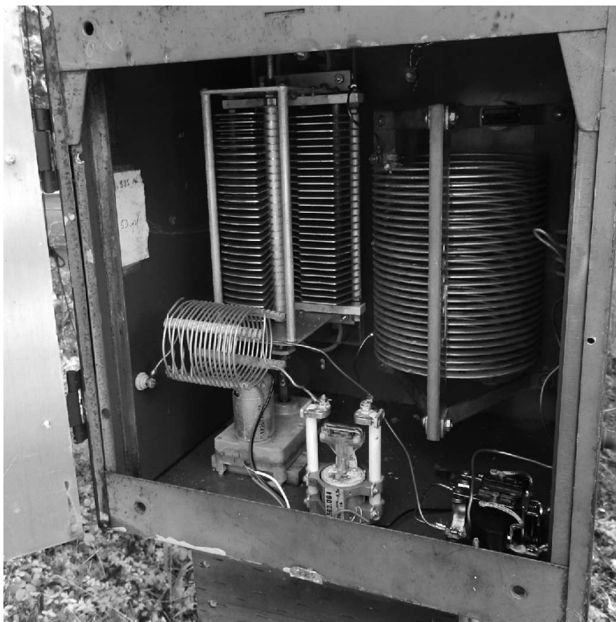
Photo 1 — This is a peek inside the parasitic loop tuning box. The high voltage surplus Russian switch is used to close the loop, thus activating the loop. A remote controlled motor-driven variable capacitor is used in series with the inductor to provide a continuously variable inductance. Thus the array can be adjusted from the shack for maximum forward gain or maximum F/B. A second lower-voltage switch is used to tap the inductor for a director pattern toward New Zealand. The director pattern is a “free feature” but is not very critical, thus fine tuning is not required. The box is an old single-drawer file cabinet with an aluminum sheet access door. The exterior of the box was painted with rust-resistance paint.
