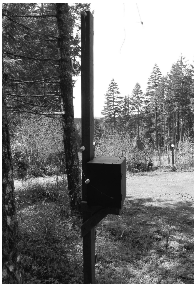
Photo H — Here is the parasitic loop tuning box, which is at the base of the east vertical element. This view is looking west down the low horizontal wire of the loop. The horizontal wire is placed about 15 feet high so delivery trucks and other vehicles can pass under it. The horizontal wire is supported by a tree in back of this view, to achieve the desired height clearance. The insulator is visible in the top left corner of the photograph.
