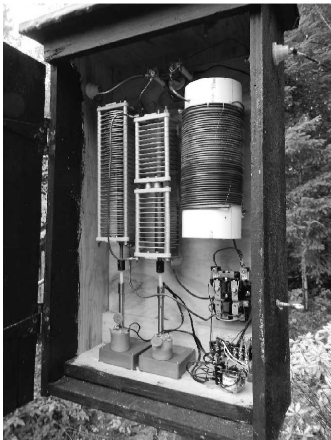
Photo G — Inside the east leg box: The high voltage switch at the top inside the box shorts the inductor out for broadside patterns. The lower voltage switch selects one of the two variable capacitors. These capacitors are in series with the fixed inductor, which is wound on a PCV pipe section. These capacitors are connected in series with the inductor and provide motor-driven variable tuning for the east and west end-fire patterns. The small relay at the bottom automatically connects the appropriate motor/capacitor for either the east or west pattern. These capacitors must be mounted on insulators. Notice also the nylon insulators connecting to the motors. The motors are 12 V DC, 6 rpm gear motors. The DC control permits easy direction changing when fine tuning the antenna.
