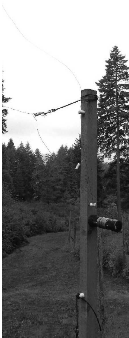
Photo J — Here is the west corner of the parasitic loop: A fixed inductor wound on a 3 inch ABS plastic pipe section with insulated #12 electrical wire solves the problem. ABS end connectors are used to close the pipe and provide a convenient mounting scheme on the post. Note the west anchor for the horizontal wire at the top of the pole using a bungee cord for stress relief. The vertical wire is fed through a ceramic electric fence insulator near the top of the post and with stress relief provided by another bungee cord. My pinot noir vineyard is in the background.
